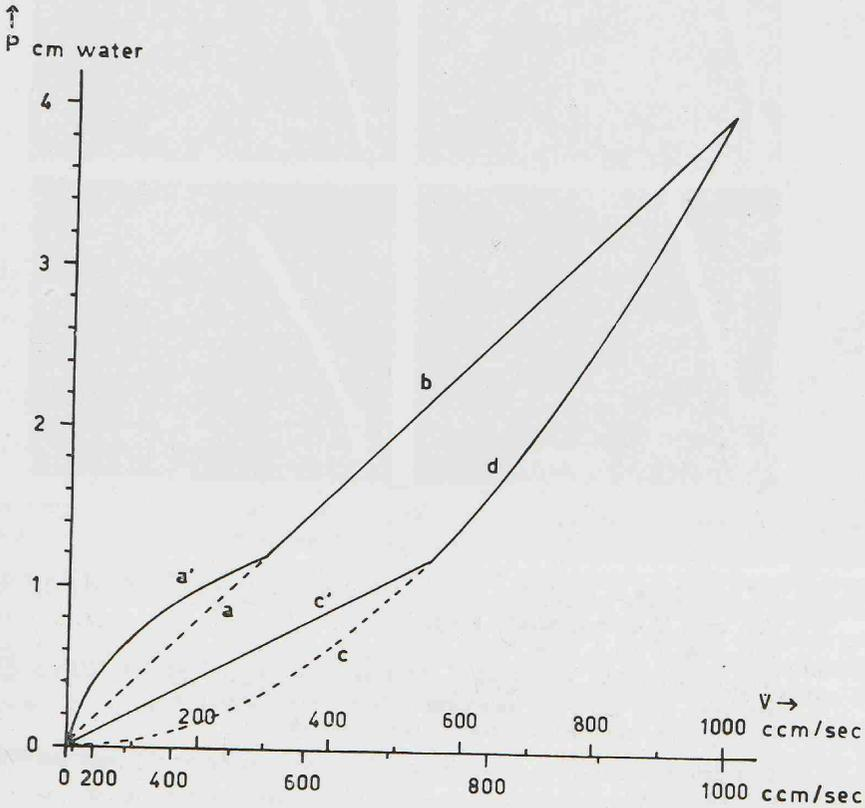
Fig. 5. The function  $P = c \dot{V}^2$  for a linear scale of  $\dot{V}$  (c and d) and for a quadratic scale of  $\dot{V}$  (a and b). Assuming that for low values of  $\dot{V}$  ( $\dot{V} < 550$  ccm per second in the drawing)  $P$  is a linear function of  $\dot{V}$  then we get  $c'$  instead of  $c$  for the linear scale of  $\dot{V}$  and  $a'$  instead of  $a$  for the quadratic scale of  $\dot{V}$ .
