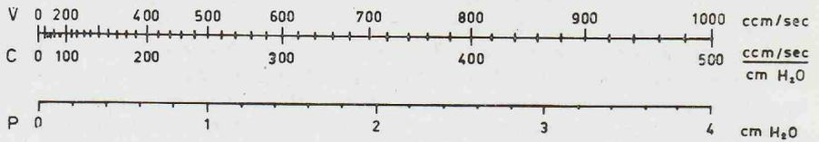
Fig. 3. Meterscales for the flow ( $\dot{V}$ ), conductivity (C) and pressure (P). The scales for the flow and conductivity are quadratic ones, the scale for the pressure is a linear one.
