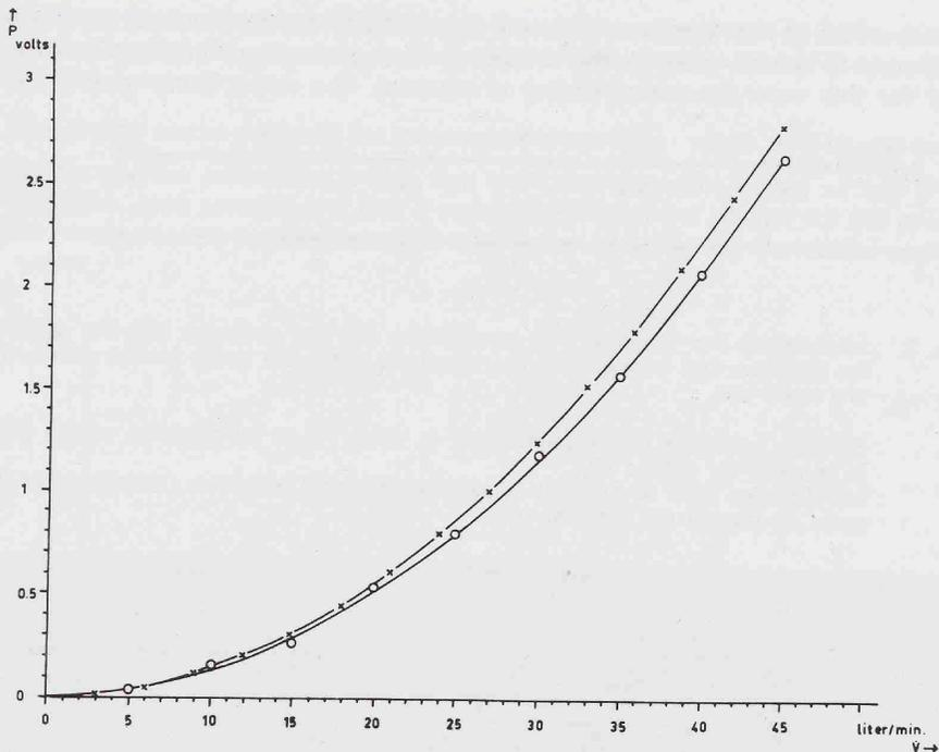
Fig. 2: Calibration of the flowmeter with a rotary flowmeter.
