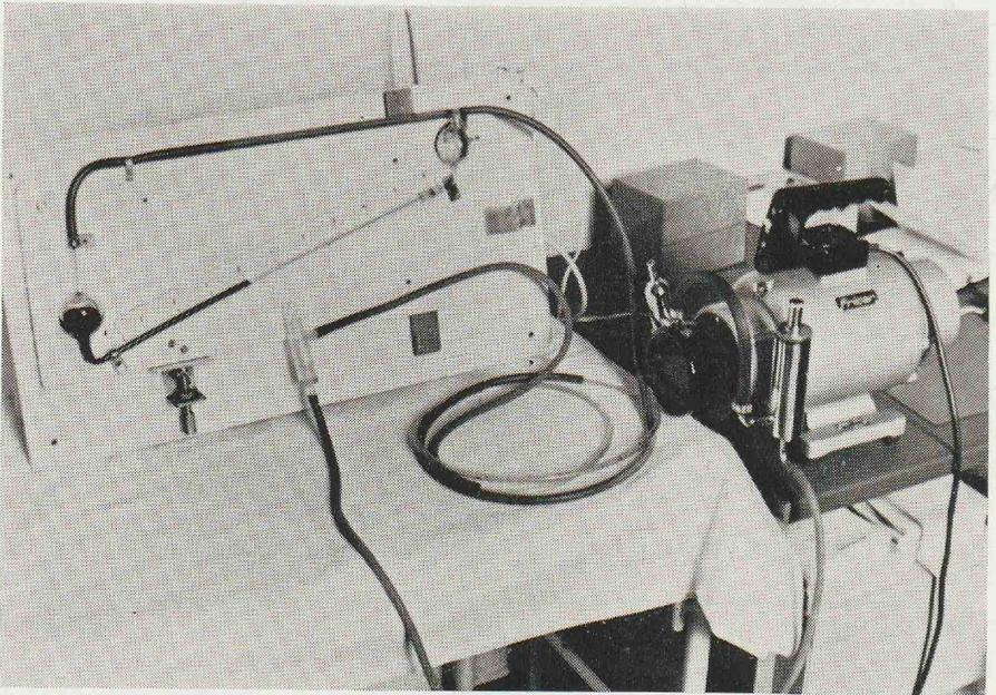
Figure A: Equipment for positive pressure passive rhinomanometry including a compressor--aspirator pump, a sensitive water manometer scaled in millimeter units on a 17 degree angle extrapolated from the vertical fluid column, and the special nozzle
