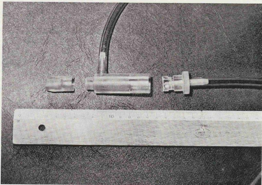
Figure C: The nozzle detail. Designed to decrease turbulence and create a more laminar flow of air.
