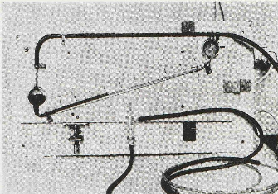
Figure B: Detail of "sensitized water manometer". The millimeter scale is spread out by being on a 17 degree angle instead of being vertical.
