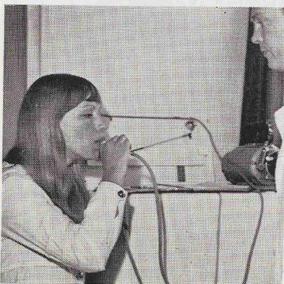
Figure G: Nasal airways tested in series. Air stream enters left nares and exits via right nares. Mouth remains closed. Nozzel tip in all testing just touches the nostril circumference creating an airtight seal. At no time does nozzel tip enter into vestibule. This prevents distortion of alae and nasal valve.
