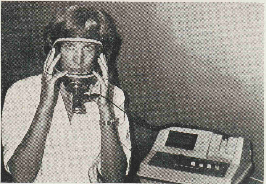
Figure 1. Examination situation: Semi-conductor transducer is fitted in opening of a panorama face-mask.
