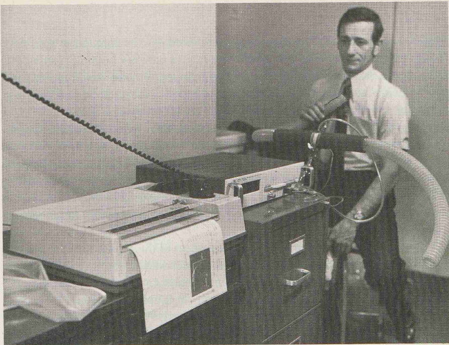
Figure 3. Results of test being received via telephone from computer center.
