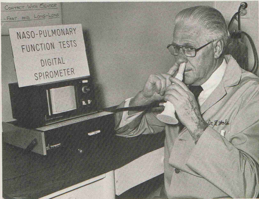
Figure 4. Testing left nose via sensor connected to digital spirometer (Life Support Equipment Corporation).
