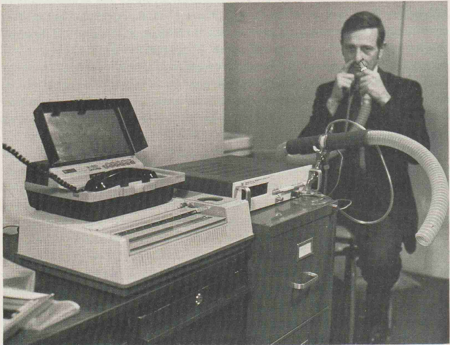
Figure 2. Nozzle in left nose leads air to pneumotachometer. Information sent to distant computer via telephone.
