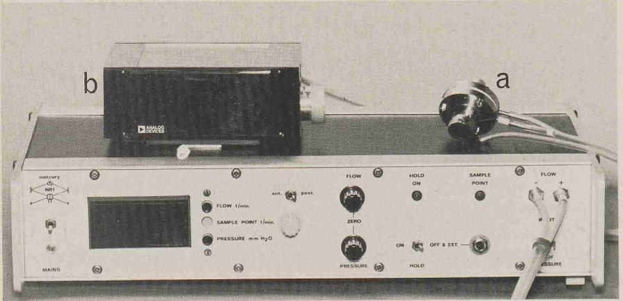
Figure 1. NR1 Nasal resistance meter. a. Flowhead. b. Extra digital display.
