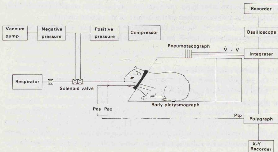
Figure 1. Schematic diagram of experimental set-up for the study of pulmonary function in guinea pig.
