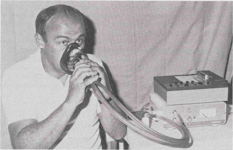
Figure 1a. The equipment manufactured by Siemens, supplemented by a pneumotachograph (interface included) and a X-Y plotter.
