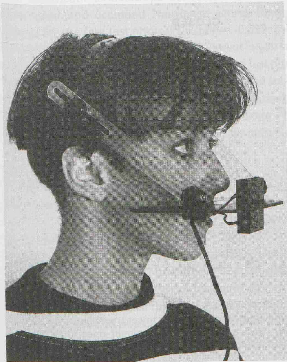
Figure 1. The Nasometer head set in position showing acoustic separator plate on which are mounted the oral and nasal microphones.
