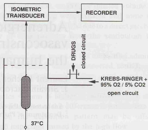
Figure 1. Experimental set-up for the study of human nasal mucosa *ex temporaneous* biopsy *in vitro*. The mucosal strip is attached to an isometric transducer in order to measure the variation of the vascular smooth muscle tension. The volume of the bath is 3 ml.
