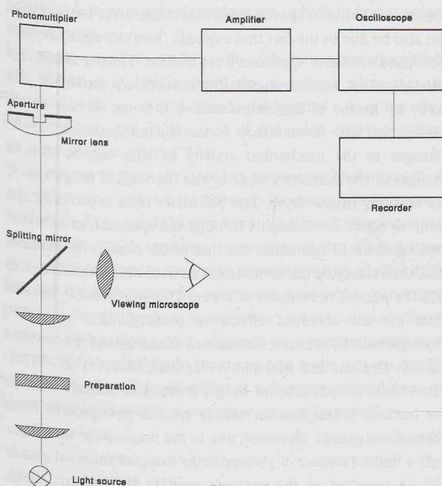
Figure 1. Schematic drawing of the experimental set-up (for details, see material and methods).
