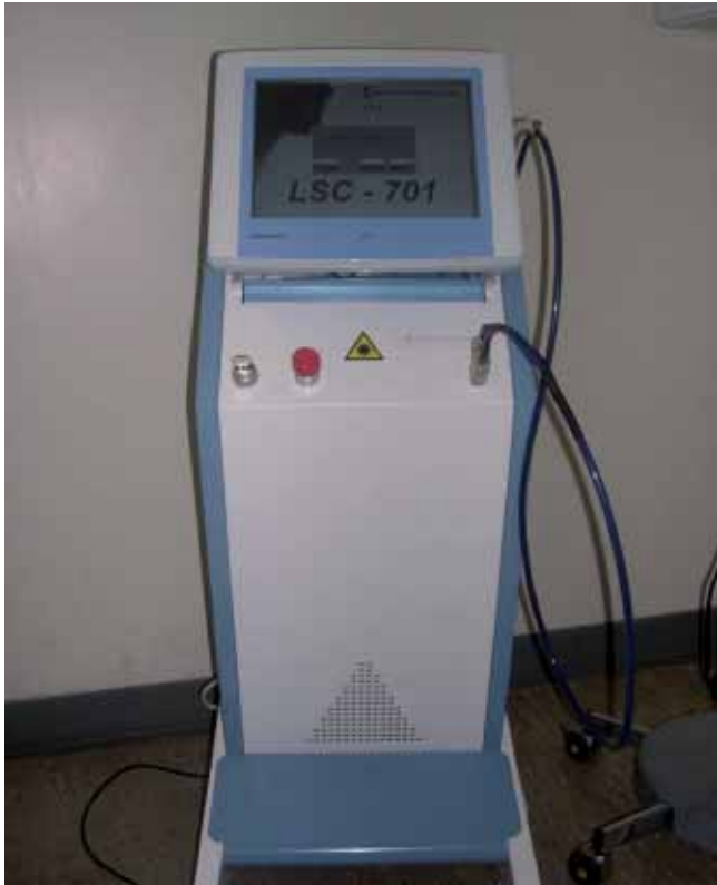
Figure 1. The Erbium doped glass fiber Laser, wavelength 1.56 \mu\text{m} and power 4.1 W (LSC-701 device - Arcuo Medical Inc).
