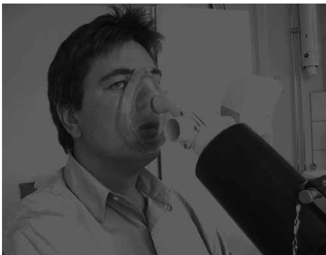
Figure 1. The study set-up: An Eco Screen ® breath condenser (Jaeger, Würzburg, Germany), fitted with a two-way, non-re-breathing valve and a saliva trap. For nasal sampling the inlet was fitted with a face mask (In-Check, Clement Clarke, England) Breathing volumes were monitored with a dry spirometer (Jaeger, Würzburg, Germany).
