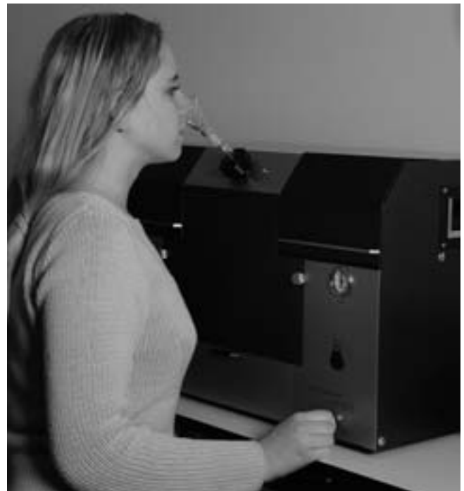
Figure 2. Measurement of the threshold level of vanilla with an olfactometer.
