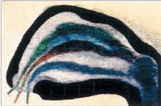
Figure 6A. Flow in a nasal model at a velocity of 15 ml/s. Parallel stream lines indicate laminar flow.
