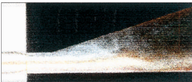
Figure 5A. Flow in a diffuser with a large increase in cross-sectional area. Onset of turbulence at the beginning of the diffuser.
