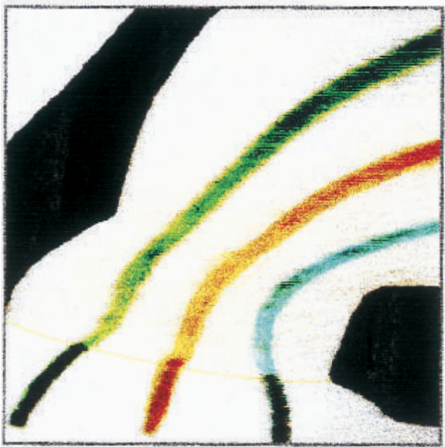
Figure 2. Flow through a nasal model. The vestibulum acts as a bend, redirecting air flow.
