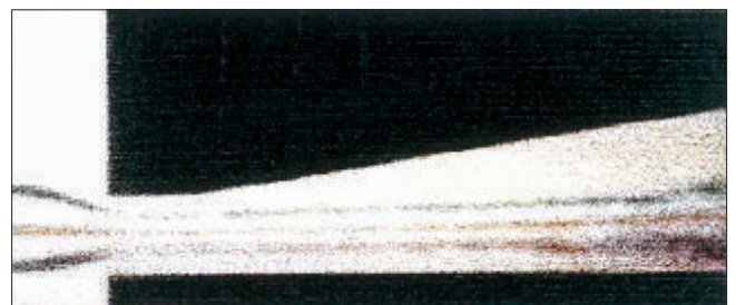
Figure 5B. Flow in a diffuser with a small increase of cross-sectional area. Onset of turbulence at the end of the diffuser.
