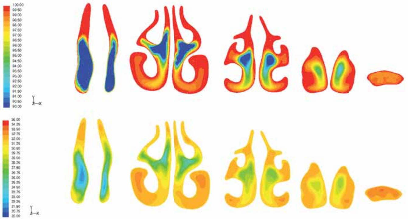
Figure 5. Humidity (upper row) and temperature (lower row) dispersion during beginning of inspiration.
